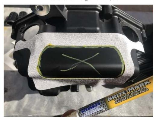
5. Install plugs into OEM airbox inlet holes.
