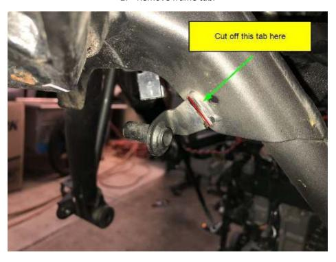
3. Install radiator mounting tab in OEM frame hole with nylon locking nut behind frame.
